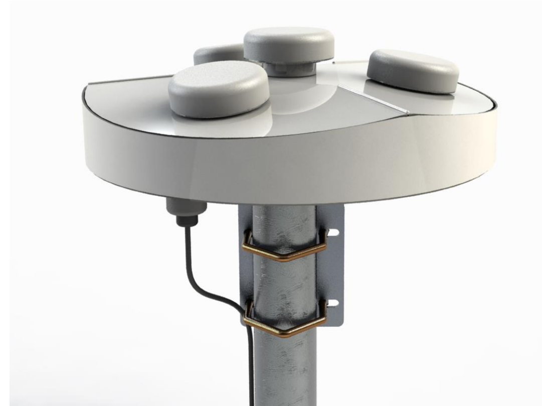
3D model of the CRPA prototype
